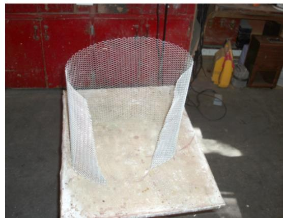
The lath is fastened together with small galvanized wire bent into a "U" shape, pushed through the pieces of lath to be fastened together and then pulled up and twisted with pliers to tighten it up. The wire will separate after a few turns or it can be cut with side cutters. Here the base diameter has been wired together to keep it together while shaping. The armature begins with a rough shape that is gradually refined. This shows the wood mandrel held in a vise used for shaping.
