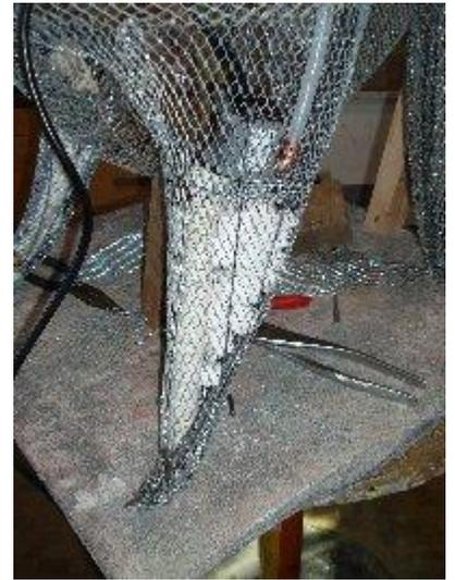
At this point, most of the upper expanded metal has been formed and fastened in place, although some remains to be trimmed and fastened to the edge wires.
